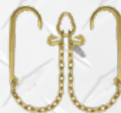
V-CHAIN ASSEMBLY 15" J hook w/ Grabs • 4,700lb WLL • Adjustable chain legs • Not for recovery P/N: N711-8 $70.99
