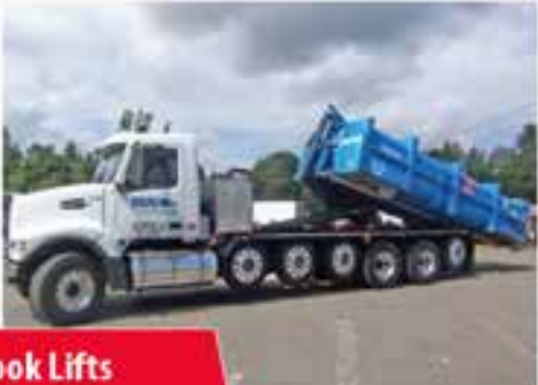
Hook Lift Trucks 400 Series Hook Lifts 33,000-40,000 LB. Capacity
